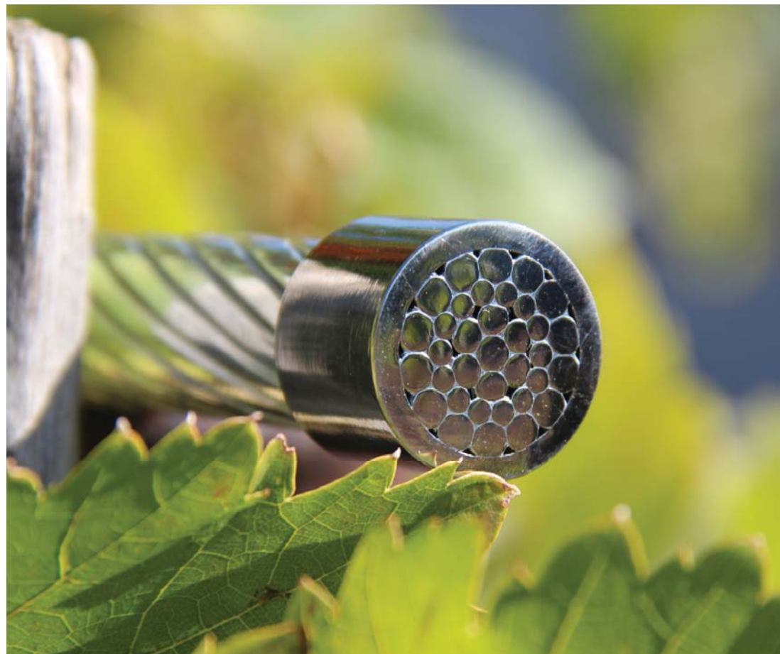
The cross section of the new Ground wire unidirectional twisted, with separate wires plastically deformed
