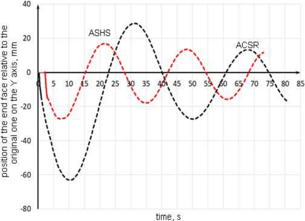
For traditional ACSR wires characterized by a significant change in the geometry of the wire in the process of oscillation with the formation of large distances between the
